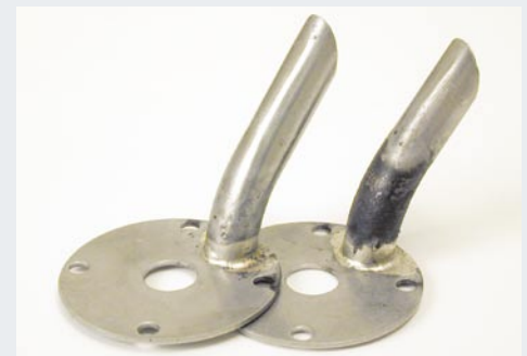
Induction brazing in a controlled atmosphere can dramatically reduce oxidation, scaling & carbon build-up.
